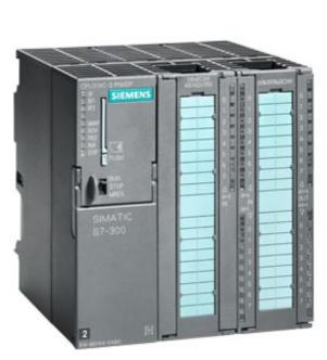
SIMATIC S7-300, CPU 314C-2PN/DP Compact CPU with 192 KB work memory, 24 DI/16 DO, 4 AI, 2 AO, 1 Pt100, 4 high-speed counters (60 kHz), 1st interface MPI/DP 12 Mbit/s, 2nd interface Ethernet PROFINET, with 2-port switch, Integr. power supply 24 V DC, Front connector (2x 40-pole) and Micro Memory Card required
