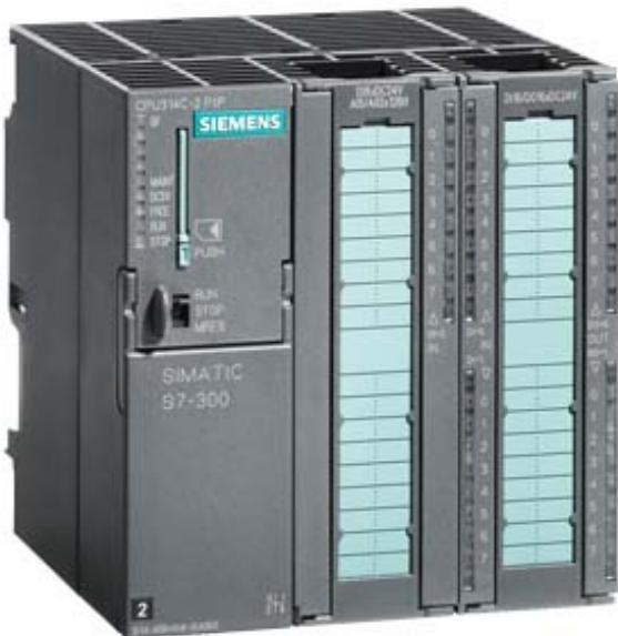
SIMATIC S7-300, CPU 314C-2 PTP Compact CPU with MPI, 24 DI/16 DO, 4 AI, 2 AO, 1 Pt100, 4 high-speed counters (60 kHz), integrated interface RS485, Integr. power supply 24 V DC, work memory 192 KB, Front connector (2x 40-pole) and Micro Memory Card required
