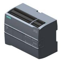
SIMATIC S7-1200, CPU 1215C, compact CPU, AC/DC/relay, 2 PROFINET ports, onboard I/O: 14 DI 24 V DC; 10 DO relay 2 A, 2 AI 0-10 V DC, 2 AO 0-20 mA DC, Power supply: AC 85-264 V AC at 47-63 Hz, Program/data memory 125 KB
